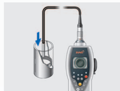
Inspection of the inside of metal parts
